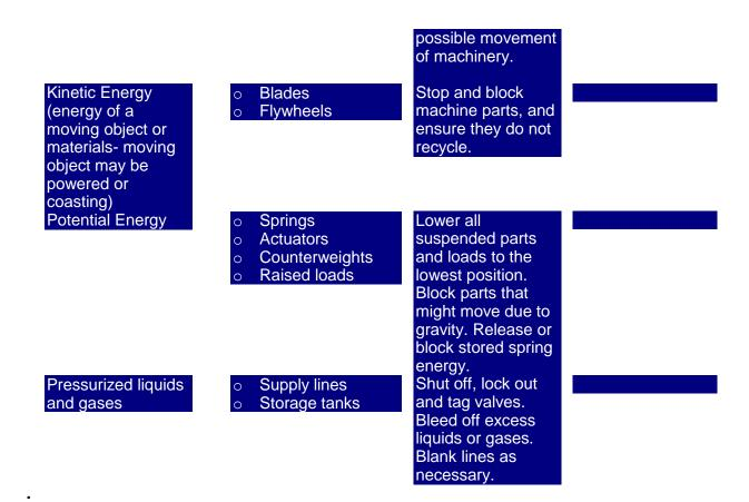
Within the Hoffman Estates Park District if equipment / machinery are equipped with a lockable electrical pull box, it will be locked out at all times when it is being serviced or worked on
